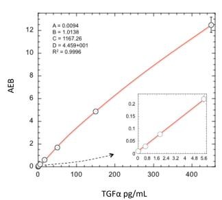
Lower Limit of Quantification (LLOQ): Triplicate measurements of serially diluted calibrator were read back on the calibration curve over 1 reagent lot across 3 instruments (5 runs total).
