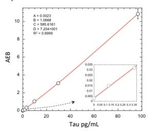
Lower Limit of Quantification (LLOQ): Triplicate measurements of serially diluted calibrator were read back on the calibration curve over 2 reagent lots across 3 instruments (12 runs total).
