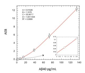
**Lower Limit of Quantification (LLOQ):** Triplicate measurements of serially diluted calibrator were read back on the calibration curve over 2 reagent lots across 3 instruments (12 runs total).
