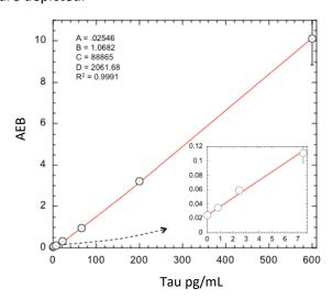
Lower Limit of Quantification (LLOQ): Triplicate measurements of serially diluted calibrator were read back on the calibration curve over 1 reagent lot across 2 instruments (5 runs total).
