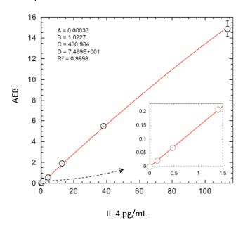
**Lower Limit of Quantification (LLOQ):** Triplicate measurements of serially diluted calibrator were read back on the calibration curve over 2 reagent lots across 3 instruments (12 runs total).
