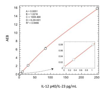
Lower Limit of Quantification (LLOQ): Triplicate measurements of serially diluted calibrator were read back on the calibration curve over 1 reagent lot across 2 instruments (5 runs total).
