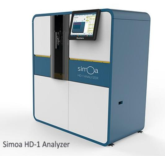
The instrument is designed to minimize operator intervention. Results are automatically calculated and can be displayed in real time upon completion of each sample's assay. The touchscreen provides the user with access to all instrument functionalities, including run setup, system status overview and result reports. The system accommodates 5 mL, 7 mL, and 10 mL primary tubes as well as 1 mL pediatric sample cups.
